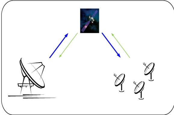
For this example, VSAT terminals are limited to 1.8m / 2.4m with 8W BUC. DVB-S2 forward (Hub>Remote) and LDPC (Remote>Hub) carrier configurations are used.
